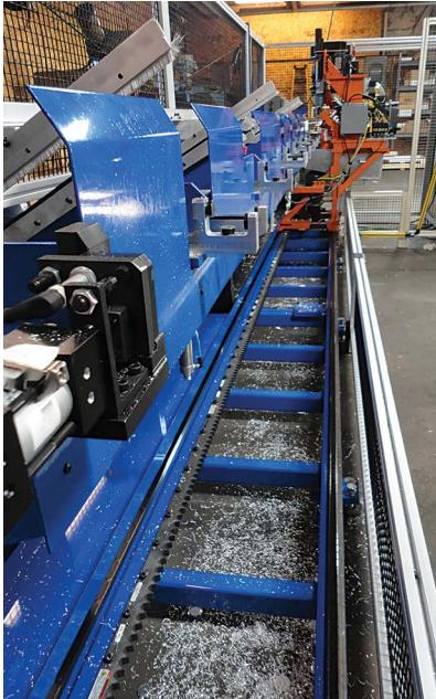
**This custom drilling and annular cutting machine makes aluminum parts for a construction-industry brake. It features a single drillhead (orange frame) that travels 16 feet at speeds of up to 2 fps. Photo courtesy Lumco Manufacturing Co.**
