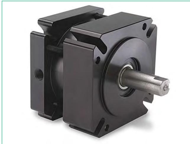
In some vertical lift applications, a servomotor drives the ballscrew. A flange-mounted servomotor brake, installed between the motor and the lift flange, will hold the ballscrew and prevent back-driving. Photo courtesy Nexen Group Inc.
