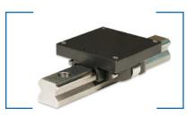
Nexen's RBR (rail brake roller) is a cost effective, light-weight solution for holding applications on guide rail systems. The unique design uses a horizontal air/spring chamber to apply force on the rail through a wedge and roller mechanism.
