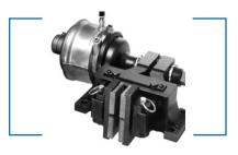
Caliper brakes are a popular design when high stopping or holding torque is required. By combining the disc diameter of your choice and one or more calipers equally distributed around that disc you can build a custom system with standard components. Caliper brakes can also be used in linear applications by clamping on a suitable rail.
