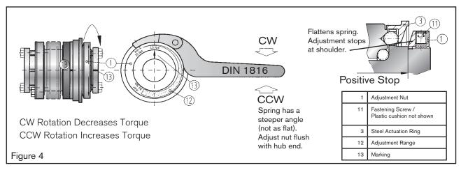
Nexen torque limiters are factory set to minimum disengagement torque within a specific range, which is marked on the MTL. The adjustment range (min/max) is also marked on the adjustment ring. The customer can adjust the disengagement torque as long as it falls into the range (12) indicated on the adjustment ring.
